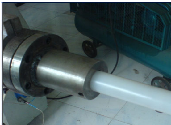
Figure 2. A photograph of extruding the pure UHMW-PE pipe with molding in barrel
